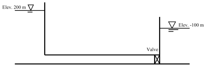
Figure 2 Schematic of the pipe system for the case study
